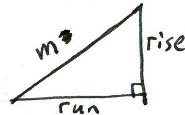
$$\text{slope } m = \frac{\text{rise}}{\text{run}}$$
