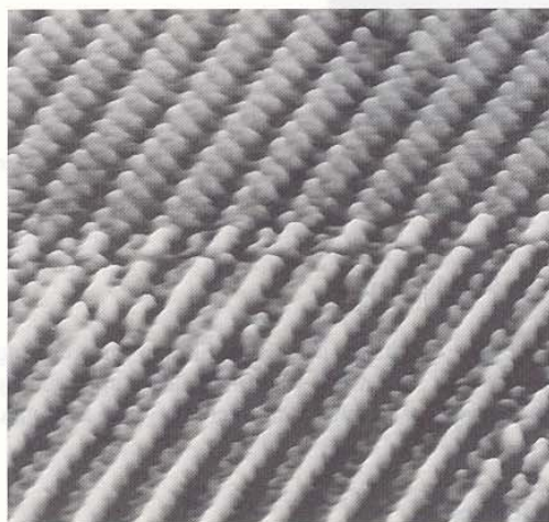
Fig. 5. A 80 \times 80 \text{ \AA}^2 STM image of \beta\text{-MoTe}_2 ( U_t = +0.3 \text{ mV} , I_t = 1.5 \text{ nA} ). Note the change from a Te-layer-like into a Mo-layer-like image.
