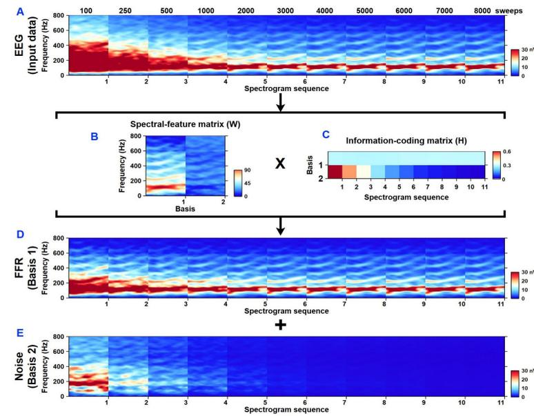
**Figure 2.** Application of the SSNMF model on EEG recordings with no silent interval. **A.** Grand-averaged spectrograms of the input data **B.** Spectral-basis matrix. **C.** Information-coding matrix. **D.** Enhanced FFR. **E.** Extracted noise.
