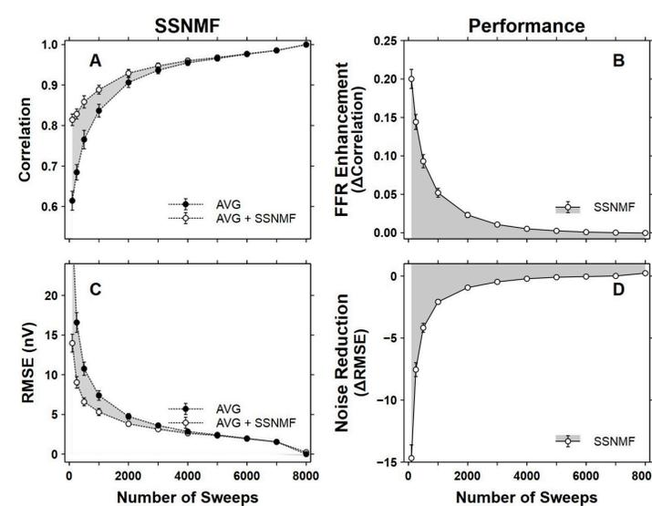
**Figure 5.** SSNMF performance with a silent interval of 150ms. **A.** Correlation coefficients before (AVG) and after (AVG+SSNMF) the SSNMF decomposition. **B.** FFR Enhancement as a function of the number of sweeps. **C.** RMSEs before and after the decomposition. **D.** Noise Reduction with increasing number of sweeps.
