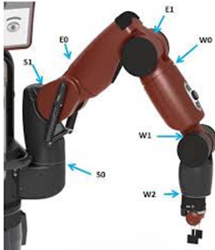
Figure 2. Baxter 7-dof Left Arm R Joints (Rethink Robotics, 2016)
