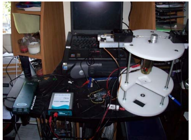
Figure 4 - Test Setup. The three white discs provided the structure for the testing. A motor was mounted on the underside of the top disc and a capstan was attached to the shaft. The two black rectangles are the force sensors and strung between them is the cord. To the left of the left sensor, the servo can be seen which applies the force.
