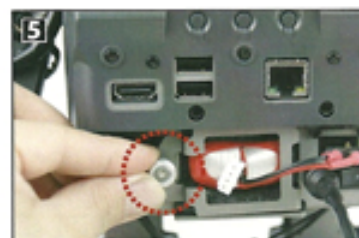
5 Insert a new battery pack and close the door
