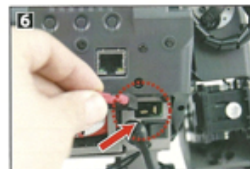
6 Connect the battery cable again
