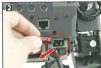
2 Disconnect the battery cable
