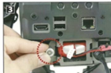
3 Open the battery compartment door
