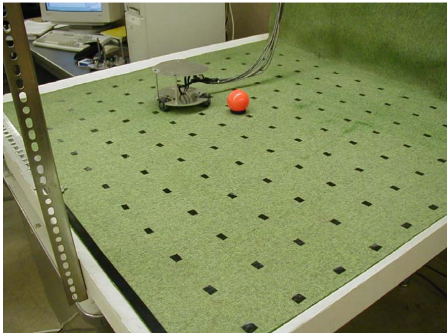
Figure 13. Experimental Setup with Omni-Directional Robot and Obstacle
