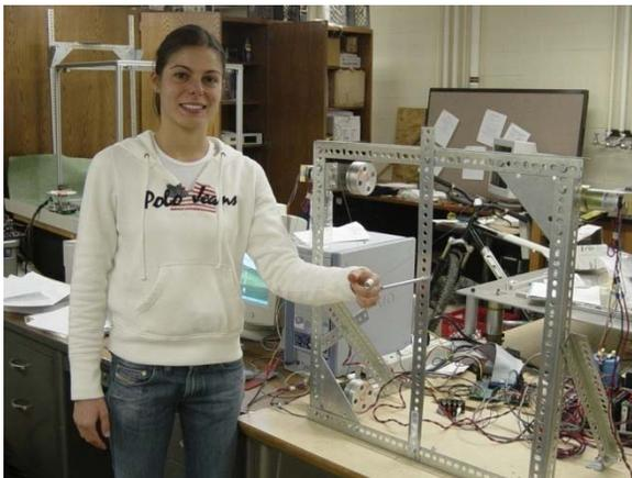
**3-dof Cable-Suspended Haptic Interface**
