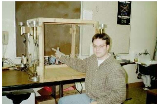
**8-dof Cable-Suspended Haptic Interface**
