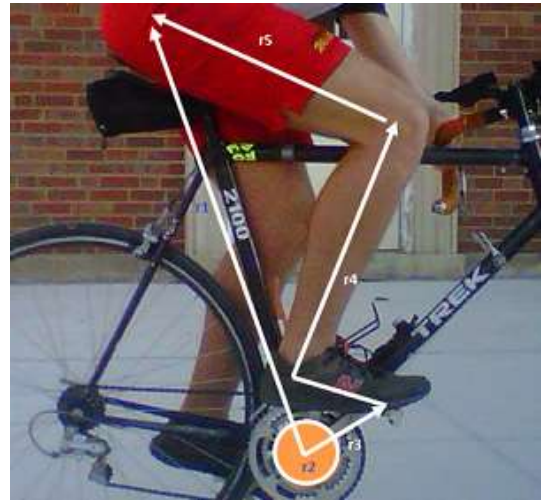
Bicycle/Human Leg 4-bar Mechanism (lock ankle)
