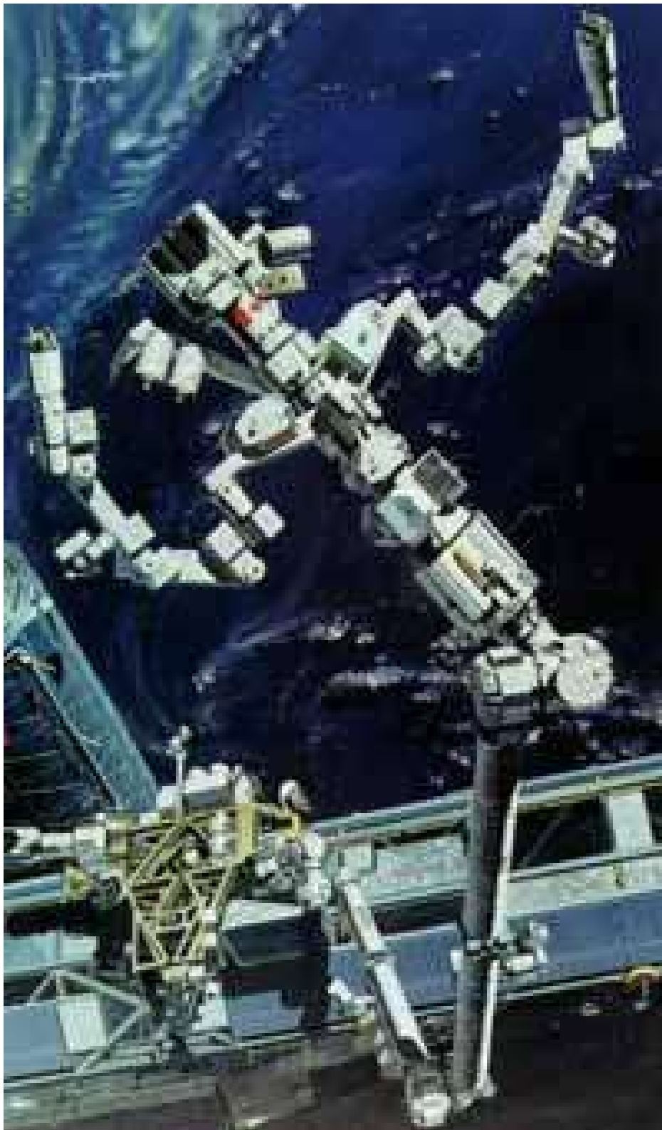
Canadian Special Purpose Dexterous Manipulator (SPDM)
